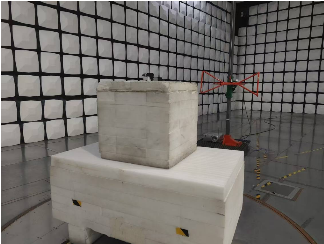
Radiated Emission Above 1GHz View
